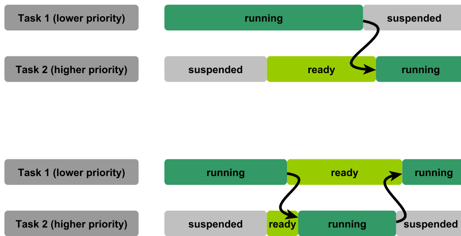
Figure 2.4: Scheduling behavior of a non (top) vs a full (bottom) preemptive task. A non preemptive task finishes execution even though a task with higher priority is in ready state. Only for certain system services, for example, an inter-process activation, the other task may be scheduled. A full preemptive task is preempted if a task with higher priority is activated. Once this task has terminated, the task with lower priority can continue running.
