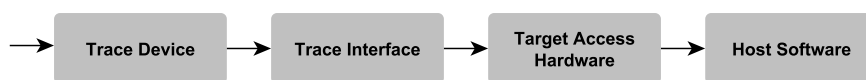
Figure 3.8: Recording a hardware trace and making it available to the user requires multiple steps. Hardware events must be measured on target via a trace device. Using a trace interface the recorded data can be readout by the target access hardware and transmitted to a host computer. Target access hardware vendors provide special software to analyze and visualize the recorded trace.
