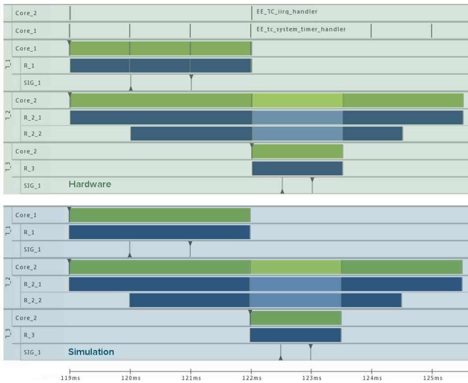
Figure 5.7: Hardware and software trace for the task-runnable-signal test model. Attention must be directed to the signal read and write accesses to SIG.1. Additionally, the nested runnables must be suspended when the respective task T.2 is preempted.
