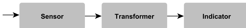
Figure 3.1: The conceptual parts of a measurement process according to Ferrari [12]. A sensor measures data. One or more transformation steps are required if the data is not yet in the desired format. Finally the result can be presented to the user.
